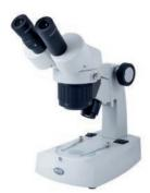
Binocular head  $45^\circ$  inclined  $360^\circ$  rotating. Widefield WF10X/20 mm eyepieces. Turret-type magnification changer (2X, 4X). 95 mm working distance. 2LBB: base with fixed arm and incident and transmitted illumination. Incident and transmitted tungsten 12V/10W illumination. Dust cover included. Supply 220-240 V (CE). 5 years warranty on optical and mechanical components. Delivery time 2-3 weeks
